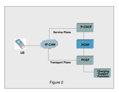
Figure 2 depicts these functions at a high level. The PCRF puts these dynamic policy rules at the edge of the network, binding the service plane and the bearer plane. It stores and acts on policy rules originated by the P-CSCF (Proxy Call Session Control Function) in the service plane. It directs and applies these policy and charging rules to the Access Gateway of the IP-CAN (IP Connectivity Access Network) where the rules are enforced.
